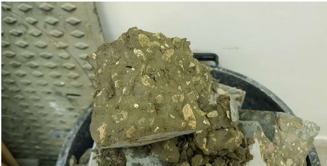
Figure 23: Crushed cube with a high level of OMWW%
