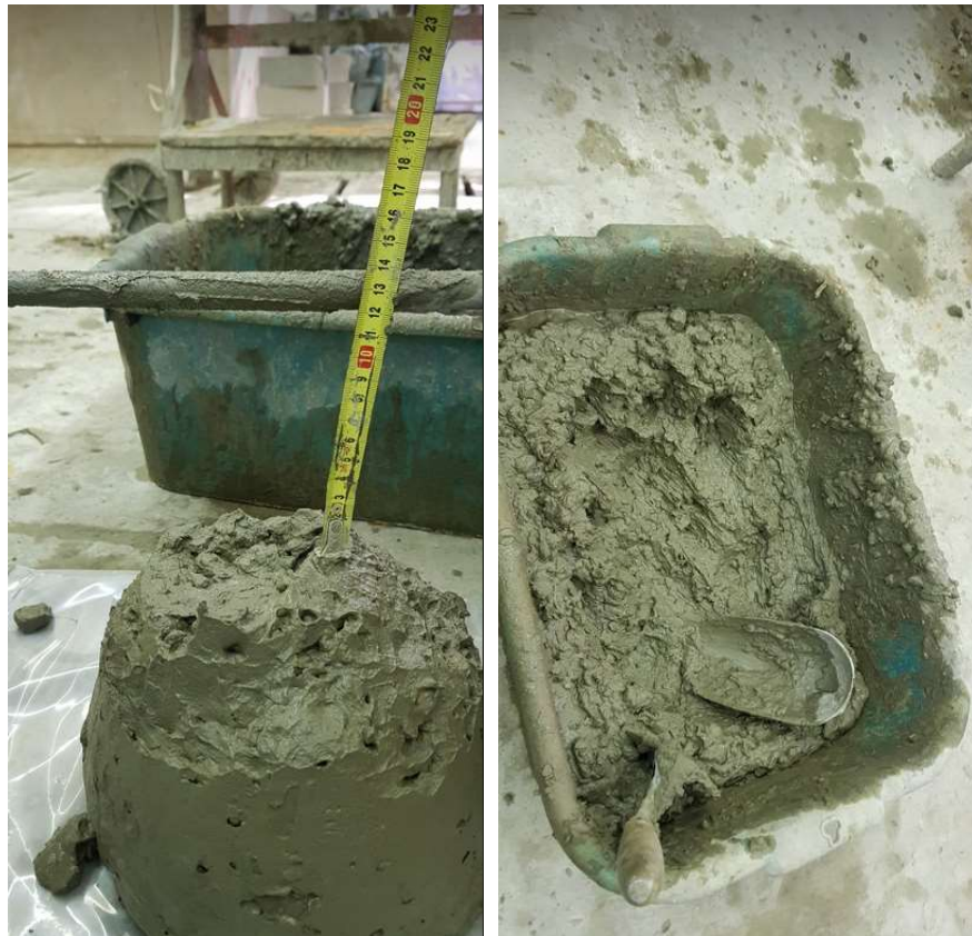
Figure 14: Concrete mix B, 12% water content, 0% OMWW, and 11.0cm slump.
