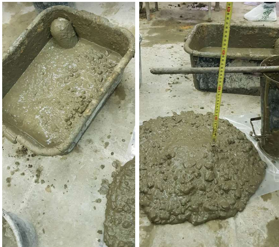
Figure 18: Concrete mix C, 80% OMWW, and 24cm slump.
