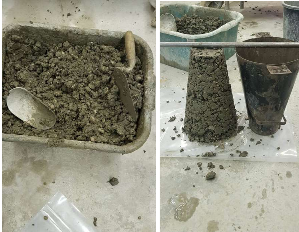
Figure 13: Concrete mix A, with 8% water content, and zero slump.
