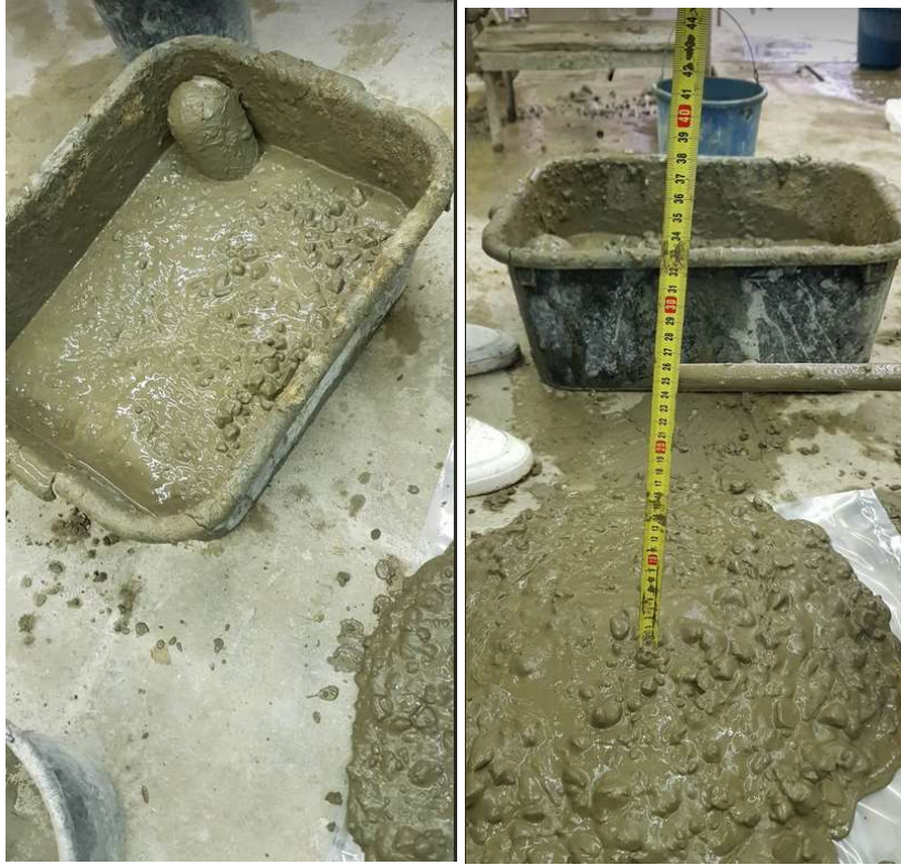
Figure 15: Concrete mix B, 40% OMWW, and 24.5cm slump
