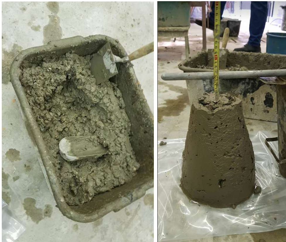
Figure 16: Concrete mix C, 10% water content, 0% OMWW, and 4.5cm slump.
