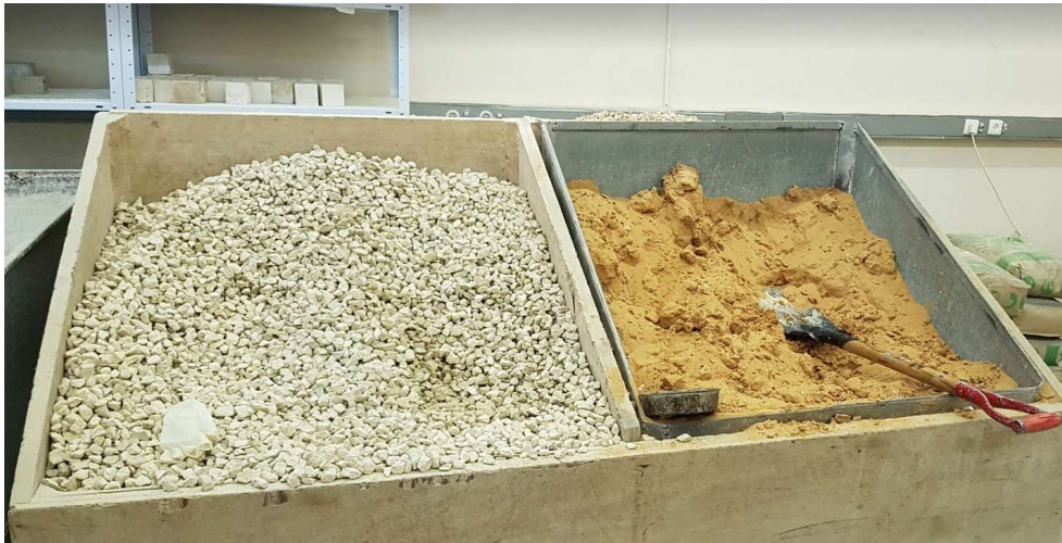
Figure 5: sand and gravel used in the concrete mixes.
