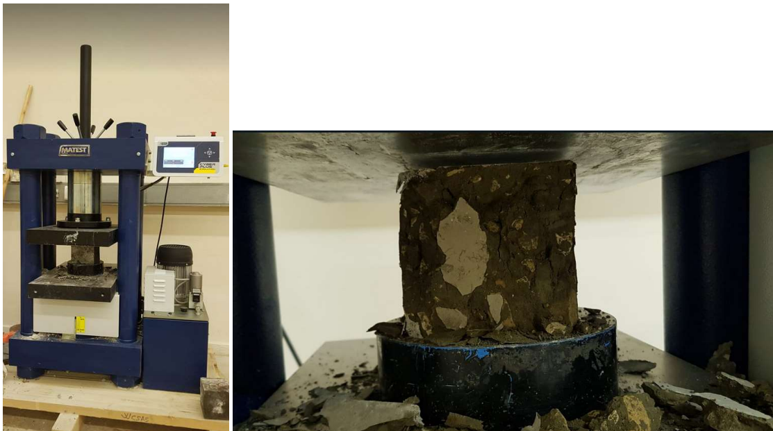
Figure 21: Concrete crushing machine and crushed cube.
