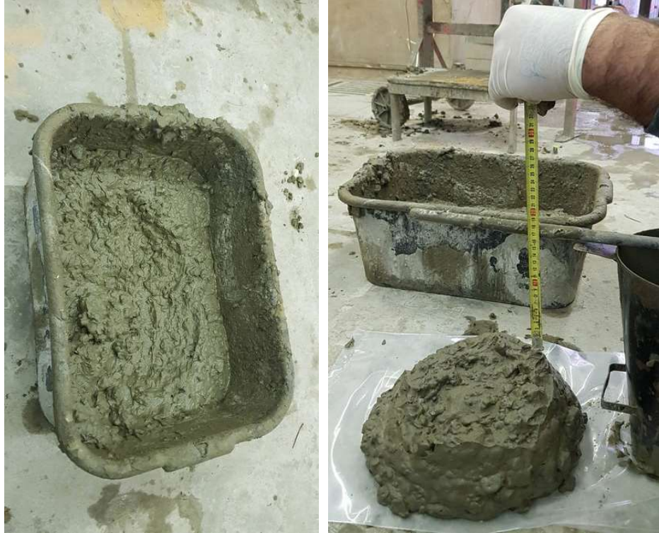
Figure 17: Concrete mix C, 10% OMWW, and 11.5cm slump
